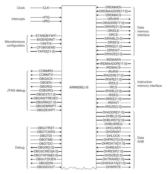
Figure 1-2 ARM926EJ-S interface diagram (part one)
