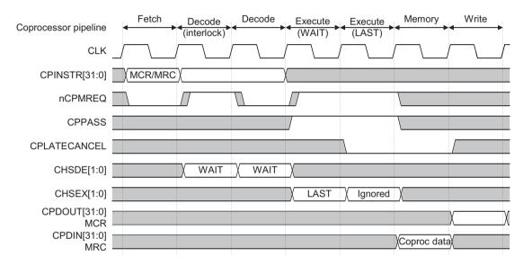
Figure 8-5 shows an example of an interlocked MCR.
