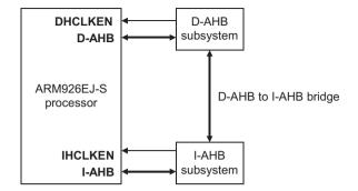
Figure 6-2 Multi-AHB system example
