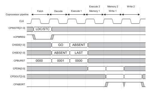
Figure 8-9 CPBURST and CPABORT timing
