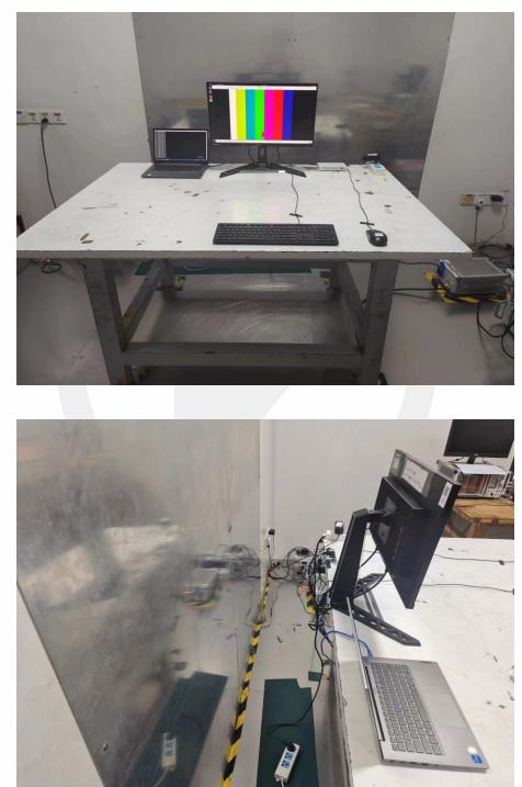
18.1.Photos of Conducted Emissions from the AC Mains Power Ports
